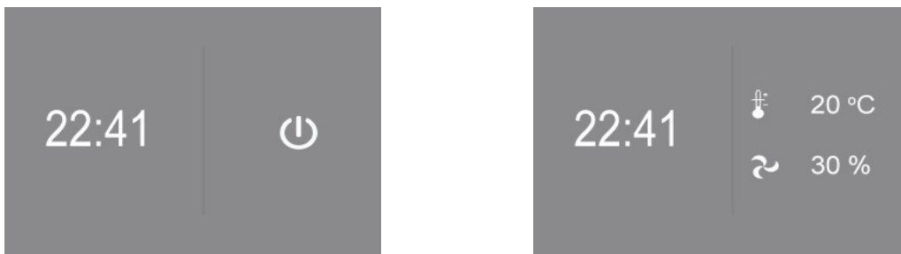
Figure 19. Control panel with touchscreen display in standby mode: the Unit is switched off, the Unit is in operation
